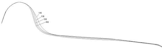
Fig. 6 Example of the wheel wear
