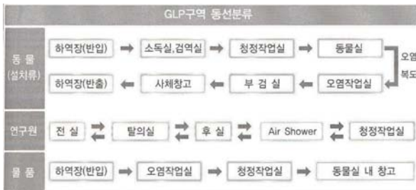
Fig. 2 Grouping of Traffic Line for GLP Area
