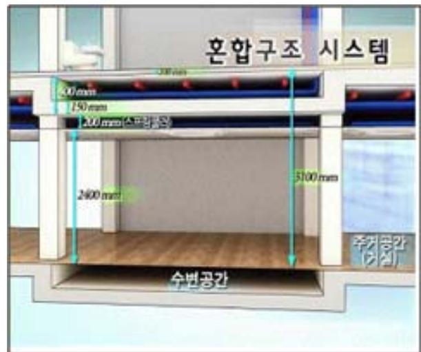
Fig. 4 Sectional Plan of Mock-Up House
