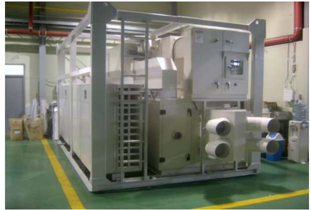
Fig. 4 Figure Picture of Four-season dedicated outdoor air handling unit (40HP).
