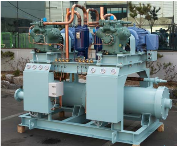
사진.2 Water cooled condensing unit
