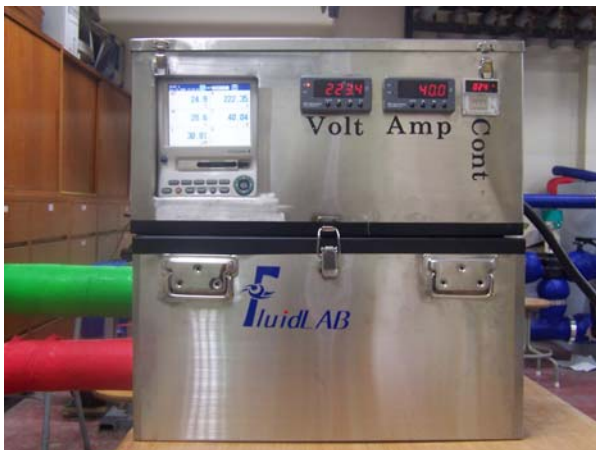
Fig. 2 Ground thermal conductivity test unit
