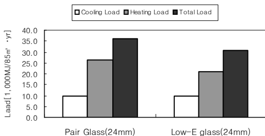
Fig. 7 Comparison of Cooling and heating load according to Low-E glass
