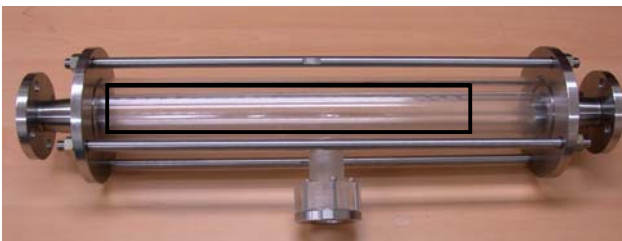
Fig. 2 IPF controller for adjusting IPF of ice slurry in a pipe: the controller consists of the outlet tube providing ice slurry and the upper tube discharging only a solution through holes).
