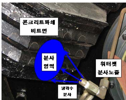
Fig. 1 Real beat plane with water-jet-impingement
