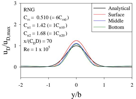
Fig. 4. Comparison between analytical and numerical solutions by the RNG  $k-\epsilon$  model.
