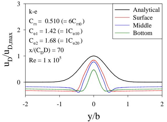
Fig. 3. Comparison between analytical and numerical solutions by the  $k-\epsilon$  model.
