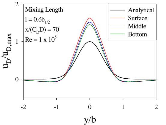
Fig. 1. Comparison between analytical and numerical solutions by the Mixing Length model.
