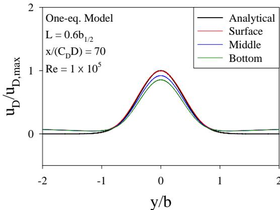
Fig. 2. Comparison between analytical and numerical solutions by the One-equation model.
