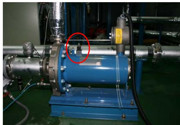
Fig. 3 Pump and vibration sensor
