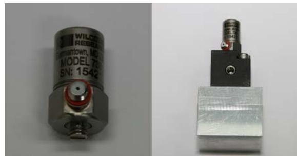
Fig. 2 Acceleration type vibration sensor
