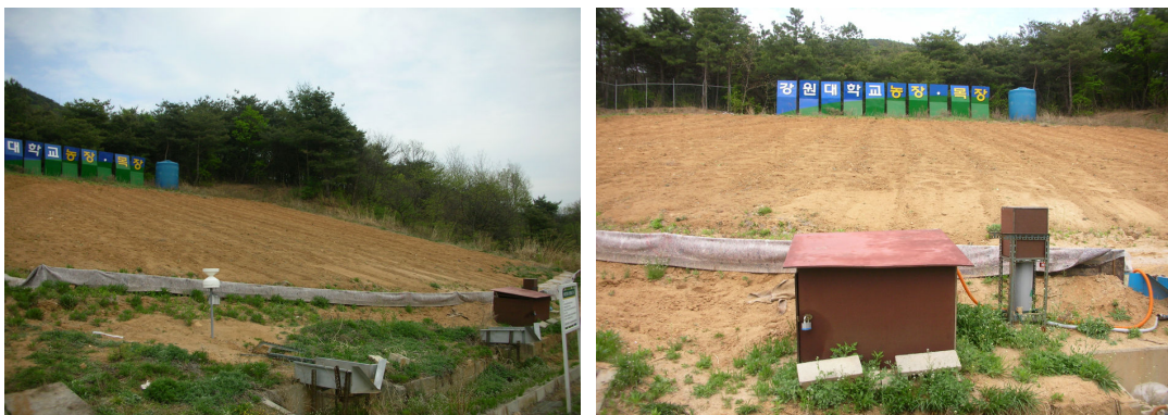
Fig. 2. View of instituted Storm-water monitoring equipment - Steep slope field.
