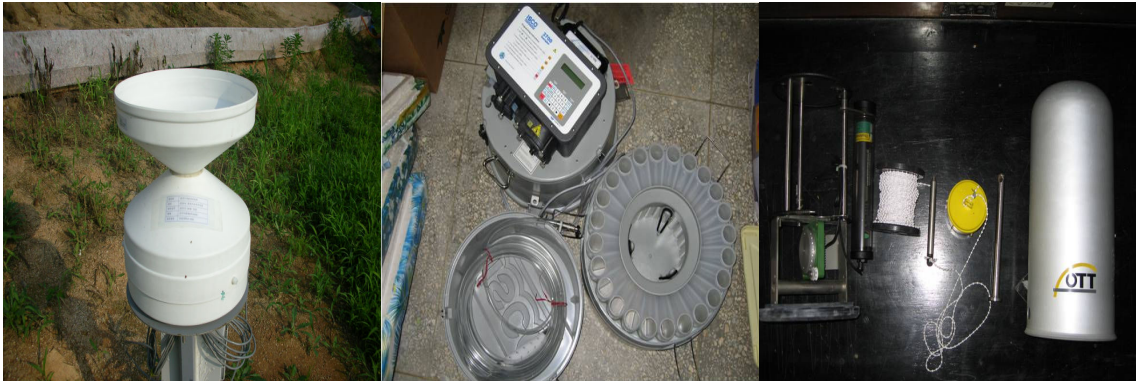
Fig. 3. Storm- water Monitoring Equipment. (a) Rain gauge (b) ISCO 3700 automatic water sampler (c) Thalimedes.
