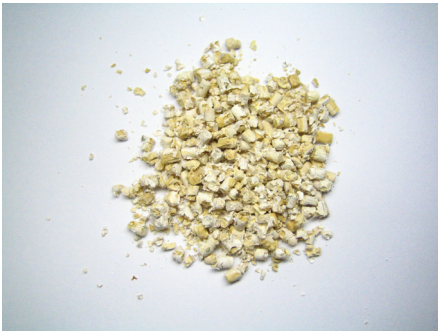
Fig. 2 Breakage of alumina pellet in high pH solution
