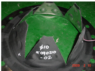
Fig. 8 Rupture Test Result
