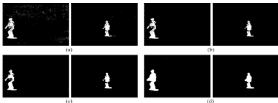
Fig. 11. Foreground mask (a), result after morphology (Open) (b), after morphology (Open + Close) (c), after NFPP (d)
