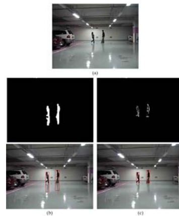
Fig. 6. (a) Origin frame, (b) The result without shadow removal, (c) The result after the proposed method applies, (parking lot)
