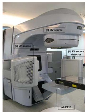
▶▶ Figure 1. The medical linear accelerator with the on-board imager mounted in orthogonal to the megavoltage beam direction
