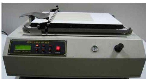
Fig. 1. Image of bar coater set up hot plate.
