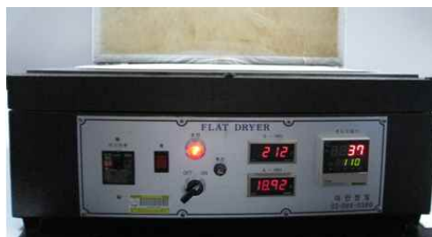
Fig. 2. Image of flat dryer used for dewaxing treatment.
