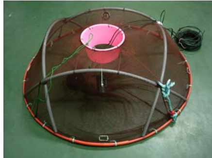
Fig. 3. The experimental pot with escape vents and infrared CCD cameras.
