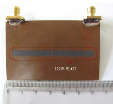
Fig. 8 Fabricated prototype of bandpass filter with DGS
