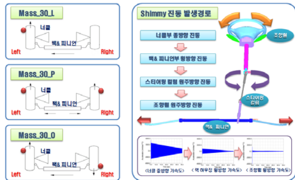
Fig. 5 Vibration transfer path of shimmy & shake
