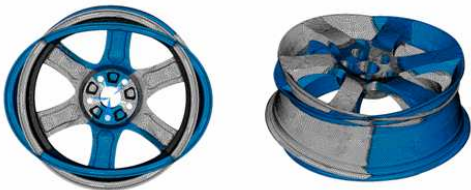
(a) rim mode (b) spoke mode Fig. 4 Mode shapes of Road Wheel
