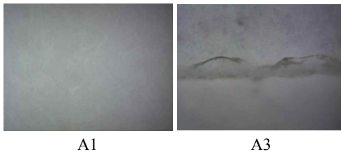
Fig. 2 Ground surface after grinding with different diamond wheel (grinding time : 30min, wheel speed : 1150m/min, material removal rate : 150mm 3 /min-mm
