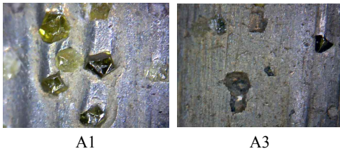
Fig. 1 Diamond grains after grinding with different diamond wheel (grinding time : 30min, wheel speed : 1150m/min, material removal rate : 150mm 3 /min-mm
