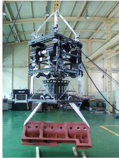
Fig. 4 The picture of the vertical moving system using a wire
