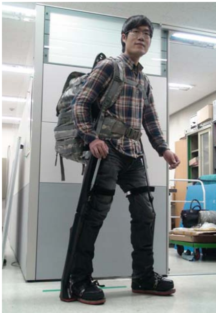
Fig. 1 Hyper-2(Hydraulic Powered Exoskeleton Robot)
