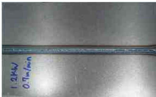
(b) Welded specimen for butt joint
