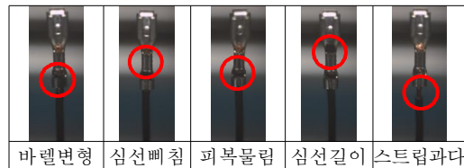
Fig. 2. Typical defective pattern
