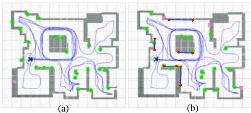
Fig. 3 Feature extraction on exploration: (a) only sonar salient features, and (b) including line features.
