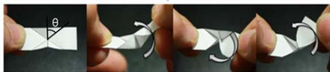
Fig.1 Paper origami trial version of SCM universal joint (a) Neutral state. (b) Pitch bending motion. (c)-(d) Yaw Steering motions
