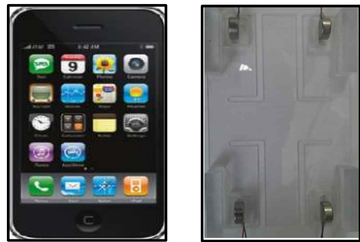
Fig. 1 Design of vibrotactile device
