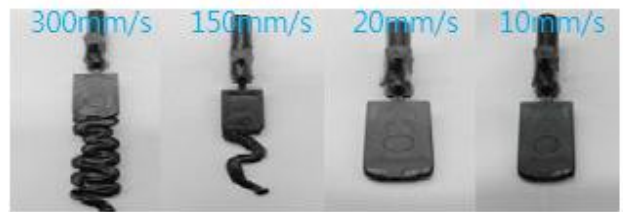
Fig. 6 Jetting of the Impact specimen according to the injection speed (C1)
