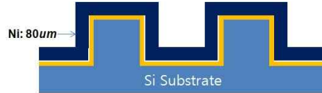
Fig. 4 Process of electroplating and seeding
