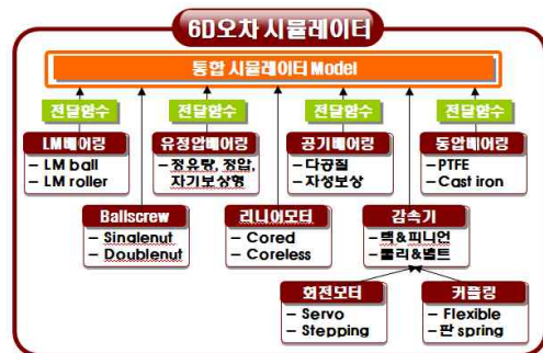
Fig. 3 Plug-in system using transfer function method for simulating the accuracy of linear motion unit
