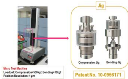
Fig. 2 Micro-Test Machine and Jigs for Fracture Tests of Korean Dentin Tissue Specimen
