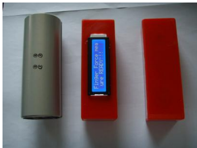
Fig. 3 Manufactured cylindrical object measuring system , LCD display and haptic device
