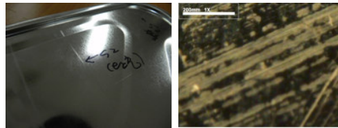
Fig. 2 Scratch on can end surface
