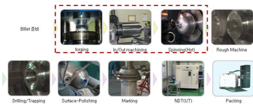
Fig. 1 Manufacturing processes of pressure vessel
