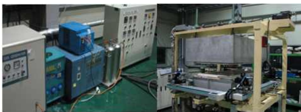
Fig. 1 Glass sealing system of experimental setup
