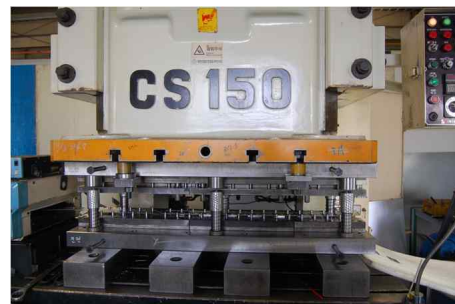
Fig. 2 Progressive die set in blanking process
