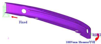
Fig. 1. Model and boundary conditions of bumper impact beam.
