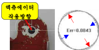
Fig. 2 Precision Measurement Results of Lug Hall
