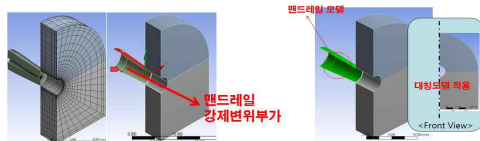
Fig. 6 FEM model applied Coldworking
