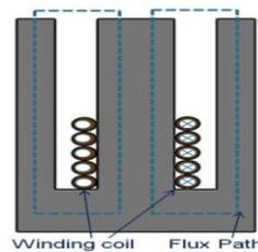
Fig. 1 Analytical Model of Electromagnet
