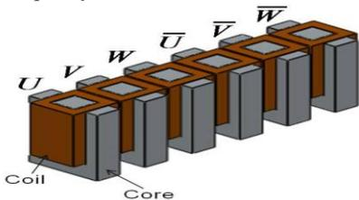
Fig. 3 Schematic Simulation Model of Levitation Actuator
