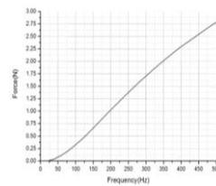
Fig. 5 Simulation result of the levitation force
