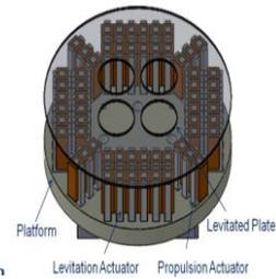
Fig. 2 Schematic Design of MPMS
