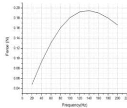
Fig. 4 Simulation result of the propulsion force
