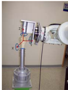
Fig. 3 Experimental Setup and Robot Tool Axis
