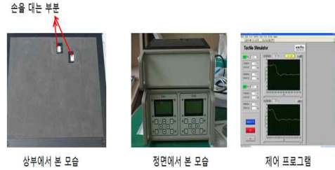
Fig. 4 Thermo display system using Peltier elements
