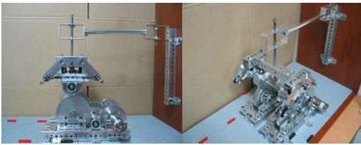
Fig. 3 Small scale wheelset roller rig- IRW type
