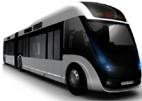
Fig. 4 The Bimodal tram showing the newly designed front part
