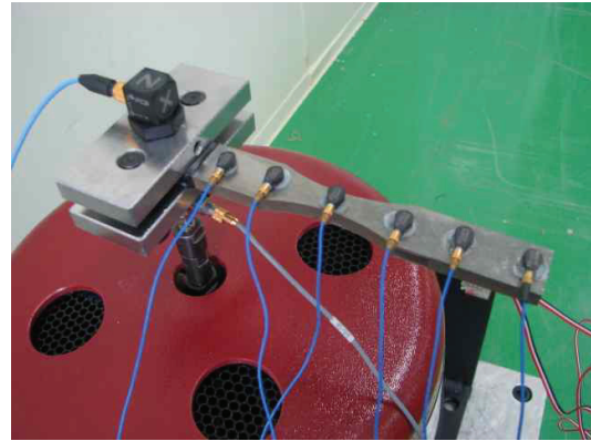
Fig. 6 Configuration of a uni-axial vibration testing
