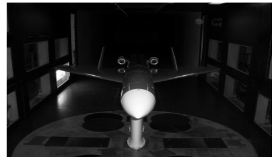
Fig. 3 The target drone for wind tunnel test
