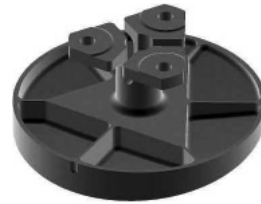
Fig. 7 Solid model of the M2 mirror
