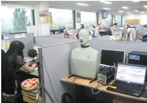
Fig. 1 Picture of measurement using HATS
